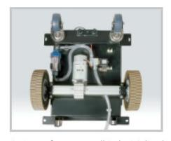
A strong frame, a well industrialized differential gear, a heavy duty electromagnetic valve and a stainless steel filter complete the machines' components.
